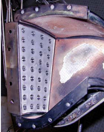
Figure 10.—A multipoint array of lean direct injectors integrated into a sector combustor rig (Ref. 15).
