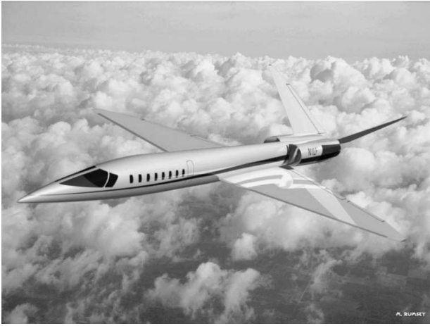
Fig. 2 Natural laminar-flow supersonic business-jet configuration.
