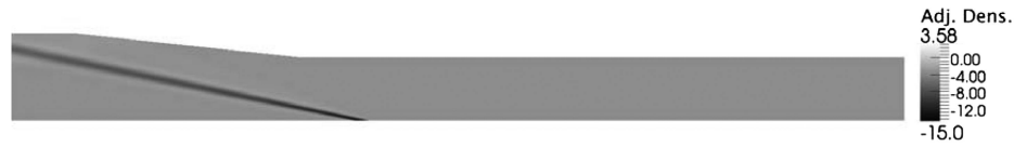
Fig. 8 Adjoint density contours for nominal conditions and pressure sensor located on the lower wall.
