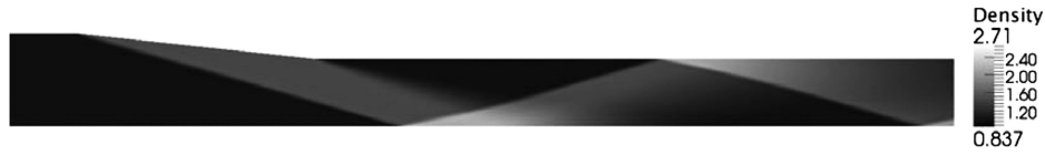
Fig. 7 Density contours for nominal conditions (inflow Mach number of 5.0 and ramp angle of 6.0 deg).
